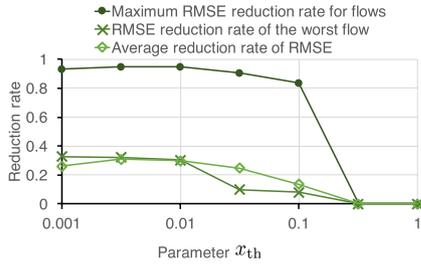
Fig. 12 Dependency of RMSE on threshold parameter  $x_{th}$ .
