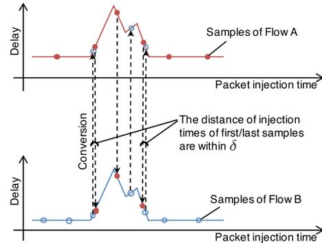
**Fig. 3** A conversion process of two flows with congestion periods that started and ended at the same time.
