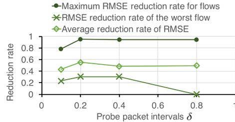
**Fig. 10** Dependency of RMSE on probe packet intervals  $\delta$ . The proposed method significantly reduces the values of RMSE.
