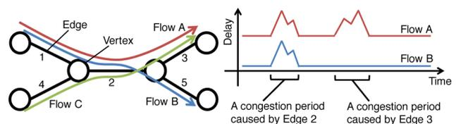
**Fig. 1** Parallel monitoring of multiple flows. The paths of Flow A and B share Edge 1 and 2. If a delay is caused by Edge 2, similar delays are observed in Flow A and B.
