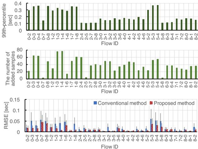
**Fig. 9** (Top) The true values of 99th-percentile of delay. (Middle) The number of the converted samples. (Bottom) RMSE of the 99th-percentile measurement for each flow.
