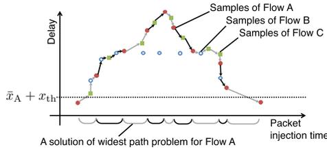
Fig. 5 Solutions of the widest path problem for Flow A.
