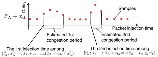
**Fig. 2** Estimation of congestion periods with samples. The threshold  $\bar{x}_A + x_{th}$  is used to estimate start and end times of a congestion period.
