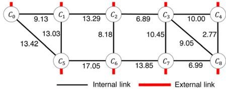
**Fig. 7** A simulation topology. The numerical values beside the links indicate propagation delays in ms.
